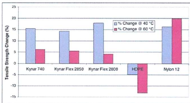
Figure 8. Tensile strength change in biodiesel with changes in temperature.
