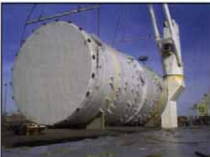
One of the scrubbers is moved onto the deck of the ship that will transport the vessels to China.
